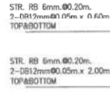
STR. RB 6mm. @0.20m. 2-DB12mm @0.05m. x 0.60m. TOP&BOTTOM
